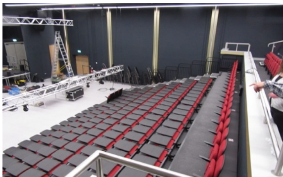
The front seven rows of seats can be rapidly retracted to provide more open floor area.
